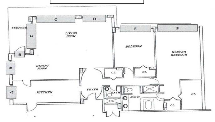
Opening Type (A): Two separate openings- Kitchen & Dining Areas: (74 x 65) Two (2) [ES1100 SH Windows] with Grey Glass with one (1) Structural Mull bar & clips
